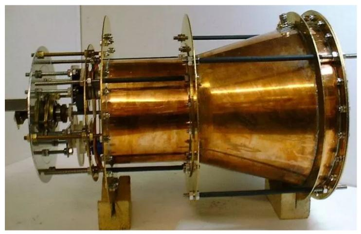
According to one peer-reviewed paper, the EmDrive thruster was able to produce 720 mN of thrust from an electricity input of 2.5 kW (Photo: EmDrive)
